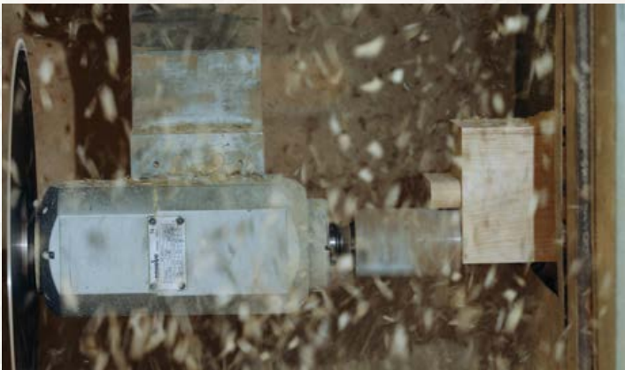
CNC Machine Milling a Tenon
