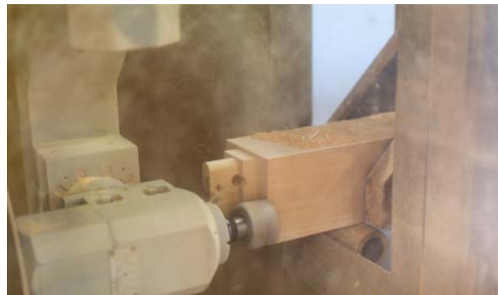
CNC Machine Shaping a Tenon
