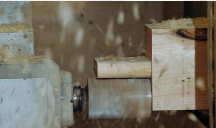
Shaping a Tenon for a Post
