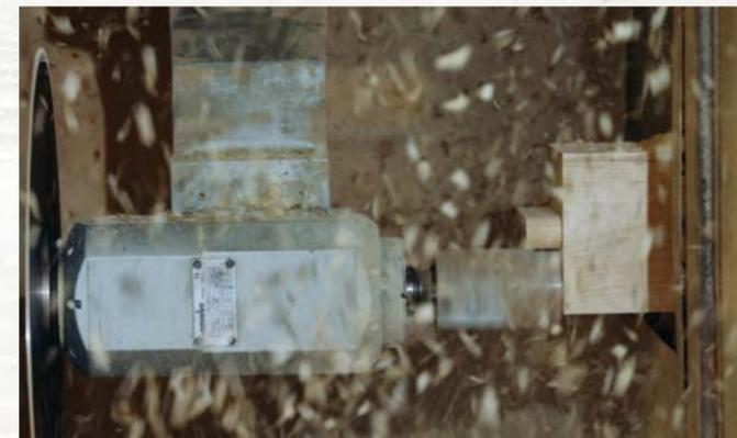
CNC Machine Milling a Tenon
