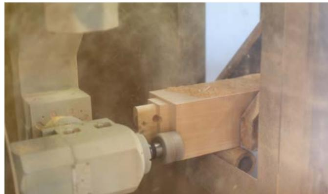
CNC Machine Shaping a Tenon
